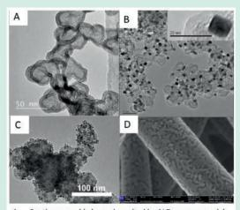
A. Continuous oxide layer deposited by ALD on commercial carbon support
